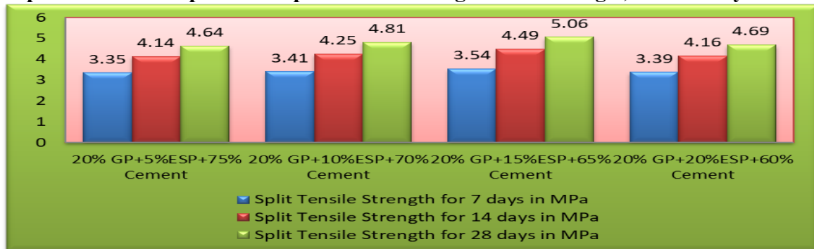
Graph No 5.4 Relation between optimum Glass powder (20%) +%ESP replacement and Split Tensile strength
