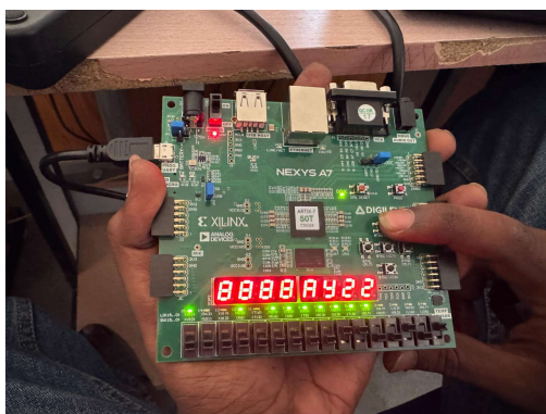
Fig. 2. FPGA Implementation – ECC Key Generation Output
