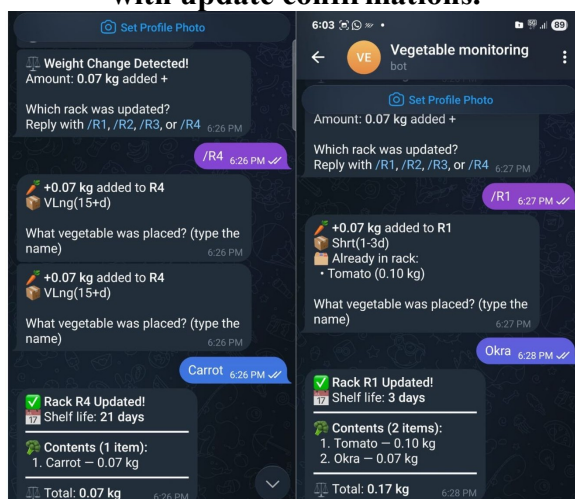
Fig. 8. Telegram interaction continued: R4 loaded with Carrot 0.07 kg (21-day shelf life); second item Okra 0.07 kg added to R1 alongside existing Tomato, demonstrating multi-item rack tracking (R1 total: 0.17 kg).
