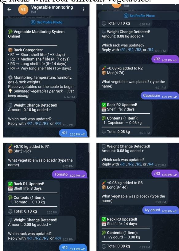
Fig. 7. Telegram interaction: welcome message with rack categories, then weight detection and assignment for R1 (Tomato 0.10 kg), R2 (Capsicum 0.08 kg), and R3 (Ivy Gourd 0.08 kg) with update confirmations.
