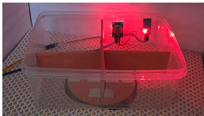
Fig. 10. Prototype in empty state: transparent enclosure, cardboard rack partitions, MQ-4 and DHT11 on interior lid, red spoilage LED active during early test.
