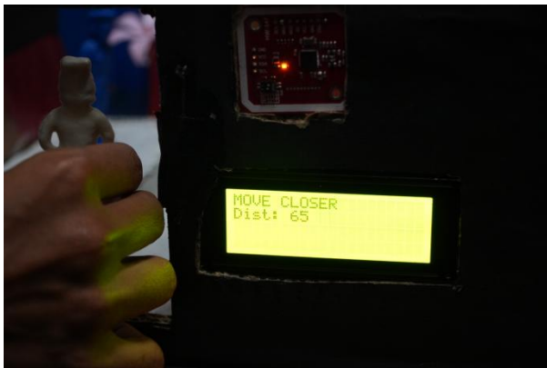
Fig. 7(a). LCD Displaying "MOVE CLOSER" with Live Distance Reading (Dist: 65 mm)
