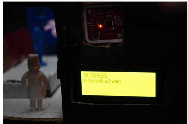
Fig. 7(b). LCD Displaying "SUCCESS" After All Three Factors Verified
