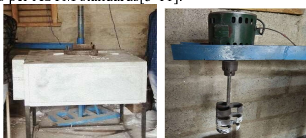
Figure 2.2 - Electrical Induction Furnace and Stirrer
