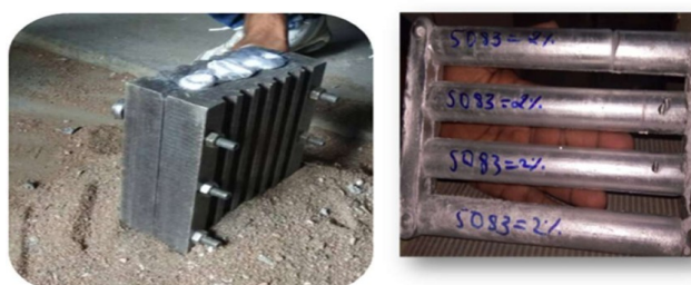
Fig 2.3 - Die used and Casted product
