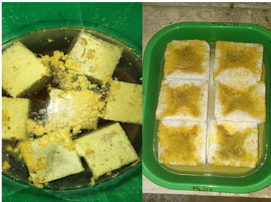
Concrete specimens under sulphate attack.
