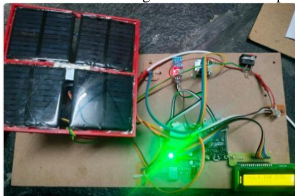
Figure 15: Realtime implementation of the device (off state)
