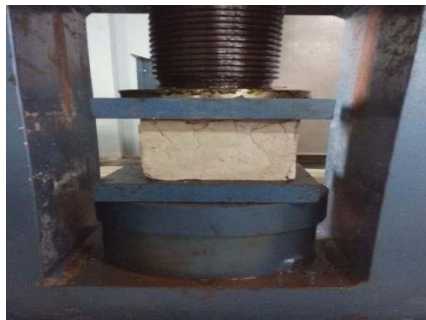
Fig no :4.5 Compressive strength test
