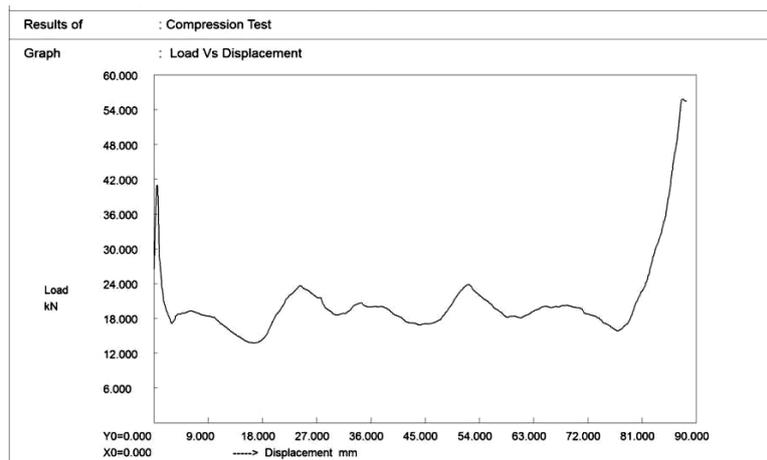
Fig. 11. Load vs Displacement Diagram for SS Circular specimen
