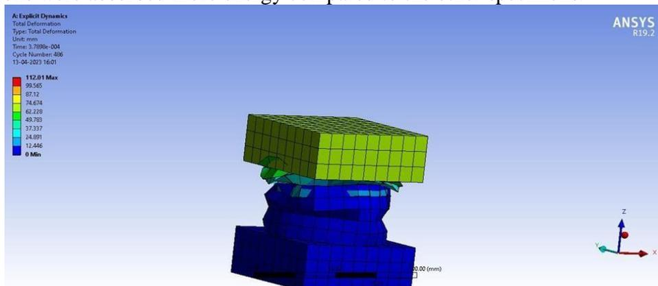
Fig. 13. GI Specimen Total Deformation
