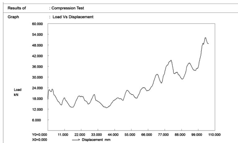
Fig. 12. Load vs Displacement Diagram for SS Taper specimen
