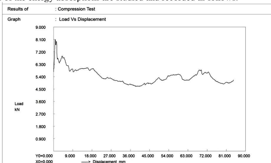
Fig. 10. Load vs Displacement Diagram for GI Circular specimen
