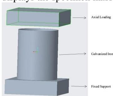
Fig. 3. Design of GI circular shape specimen
