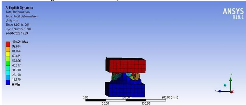
Fig. 15. SS Taper Specimen Total Deformation
