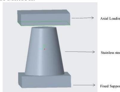
Fig. 4. Design of SS taper circular shape specimen
