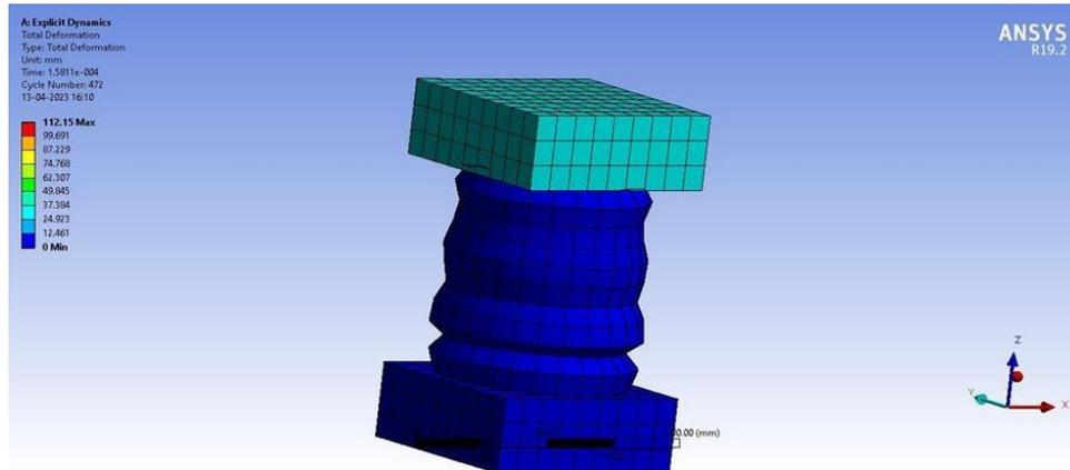
Fig. 14. SS Circular Specimen Total Deformation
