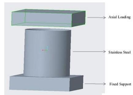
Fig. 5. Design of Stainless Steel circular shape specimen
