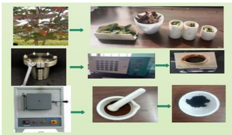
Figure 1. Flowchart of the preparation of carbon black via green synthesis followed by pyrolysis method.
