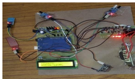
Fig 7: Count value is decremented when person exit from the boat
