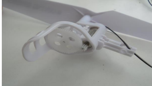
Fig: 5. Propellers Assembling to the motors
