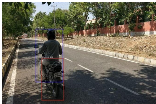
Fig. 1 (a): Frame with ‘person’ and ‘motorcycle’ classes detected (Case 1)
