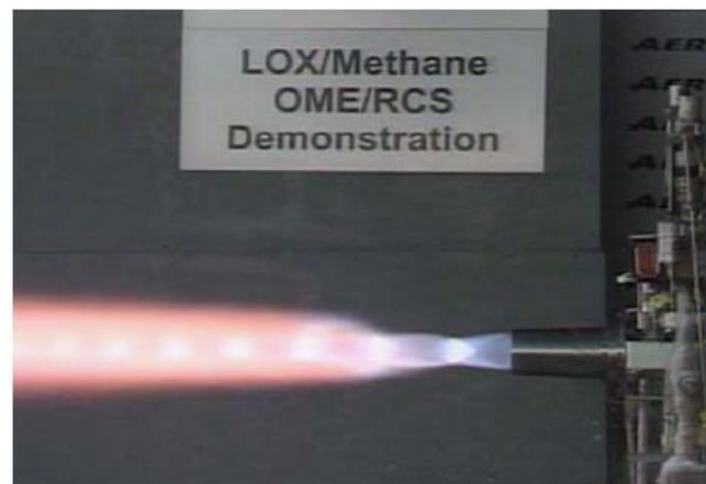
Figure 3 LOX/LCH 4 TCA hot fire testing with ablative chamber [2].
