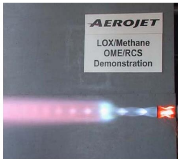
Figure 2 LOX/LCH 4 TCA hot fire test using columbium chamber [2].
