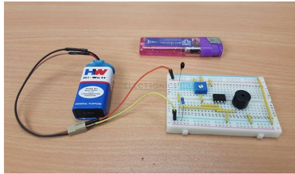
Fig. 2 : Photographic view of the developed electronic circuitry for fire detecting using bread board
