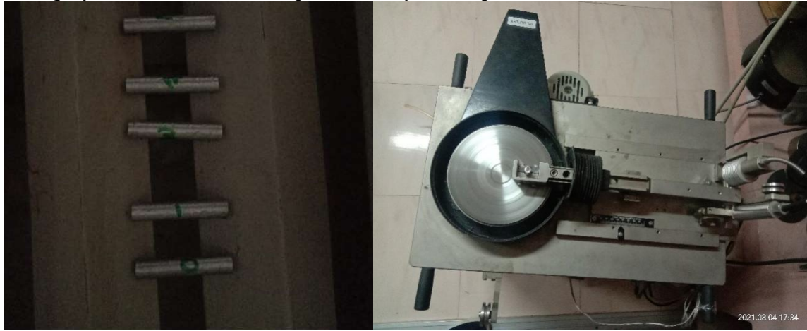
Figure 1: (a) Recycled aluminium samples; (b) Pin-On-Disc Apparatus
