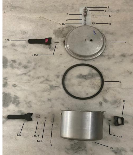
Figure 3: DISMANTLED IMAGE OF PRESSURE COOKER FOR THE NUMBER OF PARTS IDENTIFICATION
