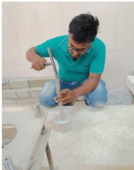
Fig. 6. Extraction of specimen from Mould
