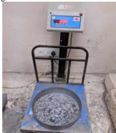
Fig. 3. Weighing the proportioned aggregates for DBM
