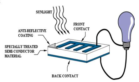
Above diagram shows performance of basic solar cell. Solar cells are made from the same semiconductor materials, that are used in microelectronic industry. In solar cells, a small semiconductor wafer is specially modified to create an electric field, positive on one side and negative on the other. When light energy hits a solar cell, electrons are released into atoms in the semiconductor space. When electrical wires are connected on both the positive and negative sides to
