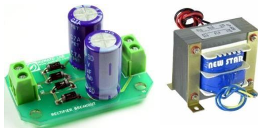
Fig.6 Rectifier and Step-down transformer
