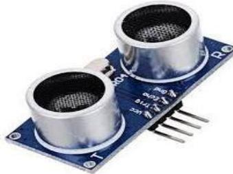
Fig 1:HC-SR04 ultrasonic module
