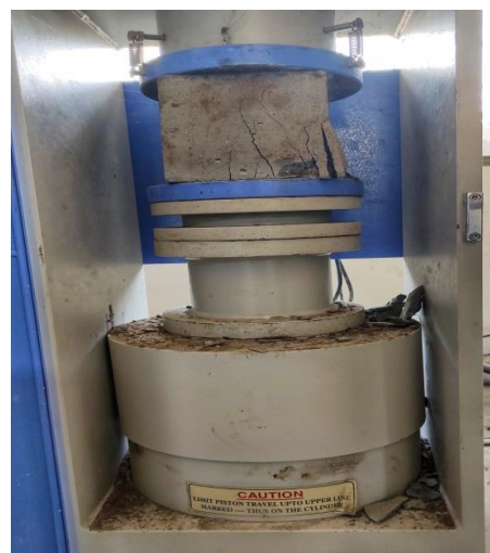
Fig-2 Testing of cube specimen
