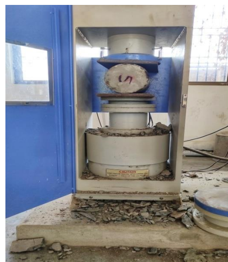
Fig-3 Testing of cylindrical specimen
