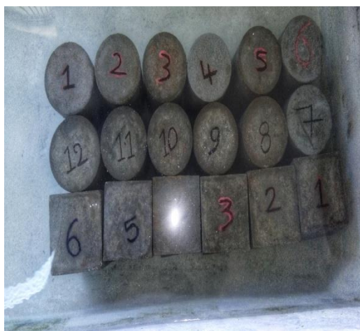
Fig-1 Samples in curing pond
