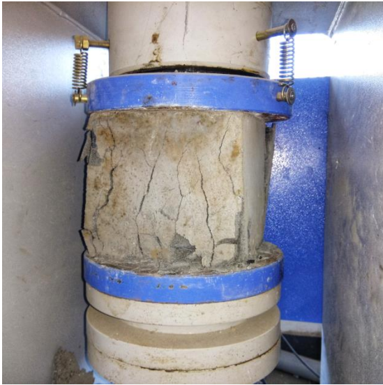
Fig – 1 Testing of cube specimen
