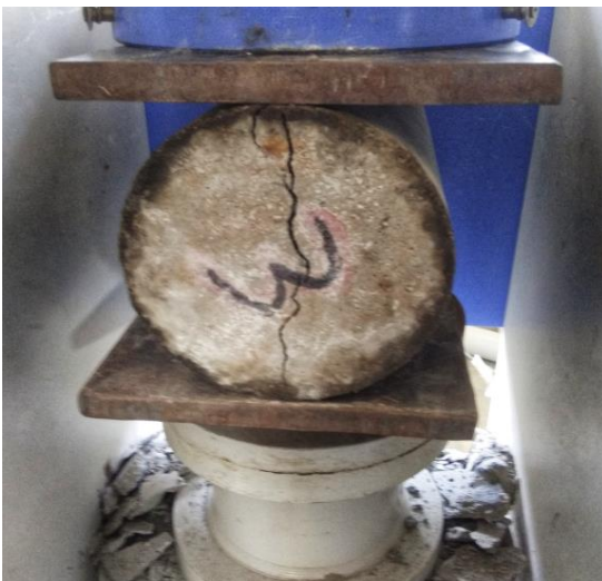
Fig – 2 Testing of cylindrical specimen
