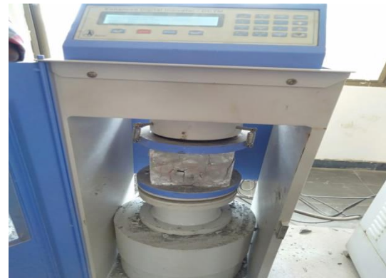
Fig.3 Testing of cube specimen
