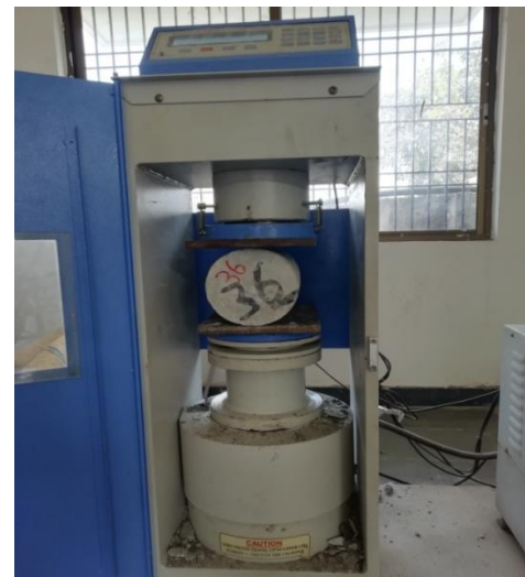
Fig.4 Testing of cylindrical specimen
