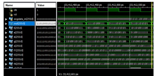
Fig 4.7 Simulation Results for Seizure Analysis of Booth Based System
